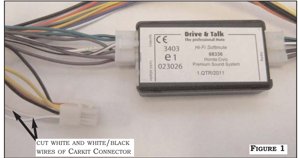
FIGURE 1: DISCONNECT CARKIT ADAPTER CONNETOR FROM BLUETOOTH HARNESS MODULE.
