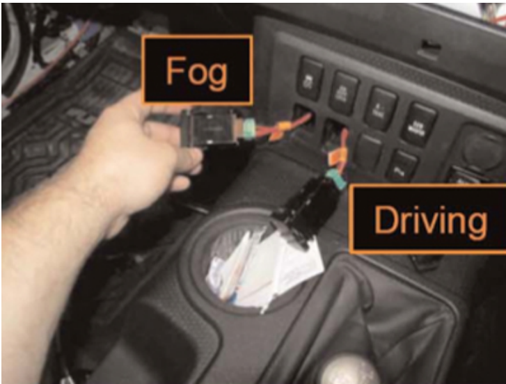
Route green Driving and Fog harness (3) plugs behind panel to connect to Driving and Fog control switches.
