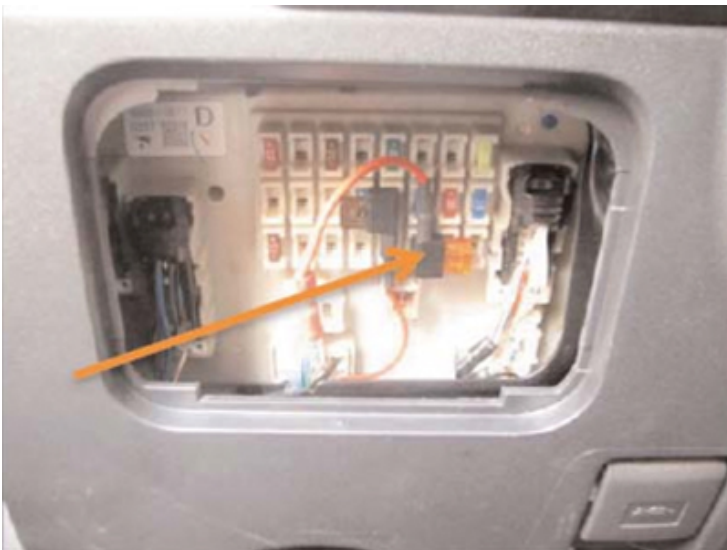
Connect the Tail light and ACC dual fuse holders to the tail lamp fuse and an accessory power circuit on the fuse panel, respectively.
