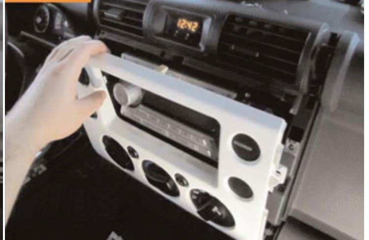
Remove radio trim by releasing upper and lower clips.
