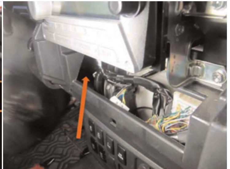
After inserting Driving and Fog lamp switches, route harness (3) to driver's side firewall area.
