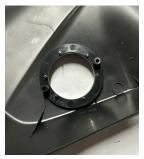
11. Using a hot knife or soldering iron, melt the plastic pins down so they secure to the black switch mounting plate. NOTE: Press firmly to ensure proper fitment.
