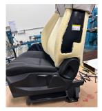
3. Separate the seat foam from the metal support bar.
